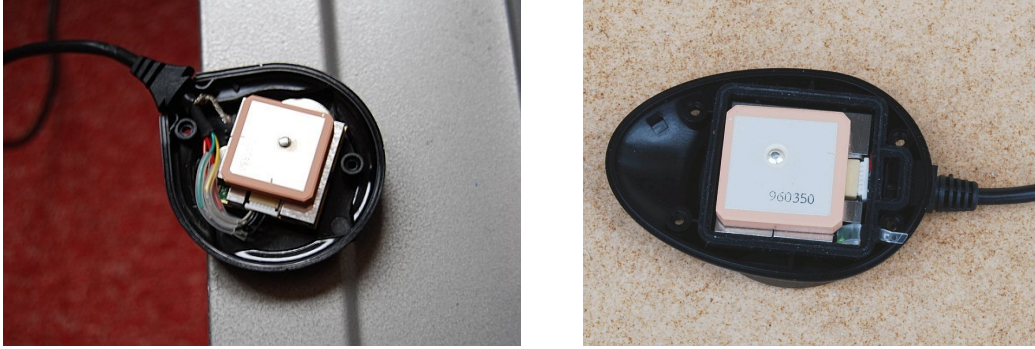
Figure 42: An EM-406A module embedded into the housing of a Fortuna U2/PS2, to the left, and embedded into a housing of a Navilock NL-303P, to the right
