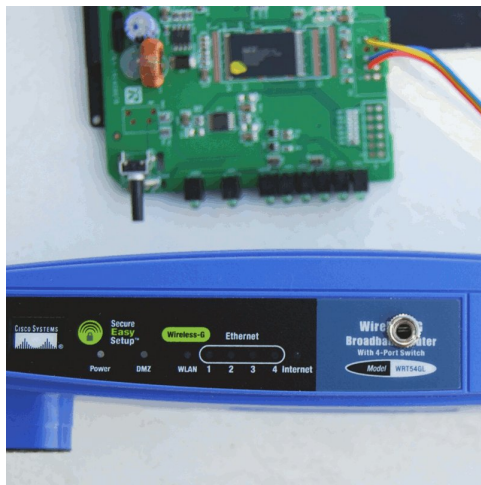
Figure 48: A modified Linksys WRT54GL router.
